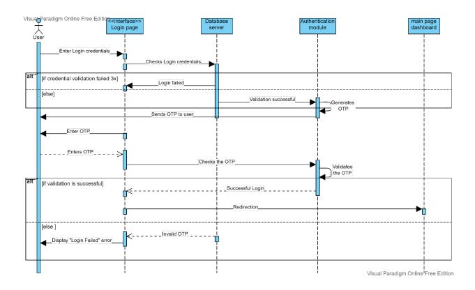
Sequence diagram showing a user who is trying to access one of the modules after successfully logging in to the main page dashboard
